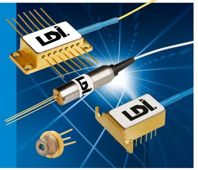
OSI Laser Diode, Inc.'s High Power laser modules are designed to meet the performance demands of the optical test equipment marketplace. The high peak optical power LCW / SCW Series lasers serve 1310nm through 1650nm wavelengths and are available in fully hermetic laser welded packages. These packaged lasers can include both TEC and temperature sensing thermistors and back facet monitors for superior wavelength stability over a wide temperature range.
