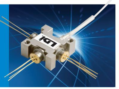
OSI Laser Diode, Inc.'s TCW TriBiner Series fiber coupled lasers are designed to meet the performance demands of the optical test equipment marketplace. These high peak optical power lasers serve 850nm through 1550nm wavelengths and are available in a compact triplex package. The TriBiner incorporates a 650nm red laser for convenient fault finder capability.
